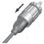
3. Rotate the large nut to tighten the plug against the receptacle. **HAND TIGHTEN ONLY.**
