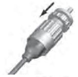
5. Rotate the red nut until it is snug against the larger nut. **HAND TIGHTEN ONLY**
