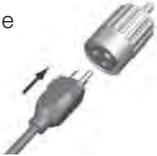
2. Slide the large nut forward to engage the threads on the plug.
